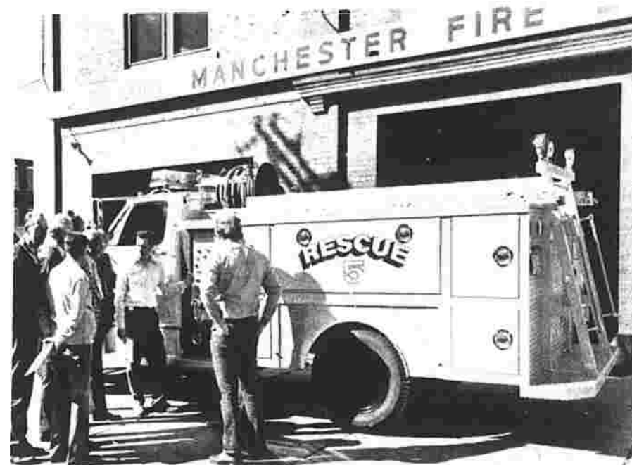
Men of the Eighth District, Chief Ted Lingard in the center facing out, get their first look at Rescue 5, a rescue and attack pumper truck. All the department's rescue gear is now stored on it for use at accident scenes. Its 500-gallon water tank enables it to put out small fires. From now on it will be the first vehicle out. In minor cases known in advance, it may be the only vehicle to leave the station. (Herald photo by Pinto)
